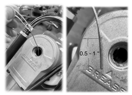
Figure 2 - Checking Grease
