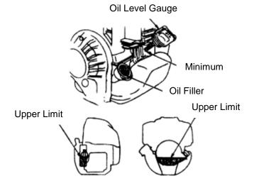
The recommended environmental temperature range of the machine is 5° to 105° F. We recommend the use of SAE 10W-30 engine oil, which equals to API classification SJ. See SAE Engine Oil Consistency Table below.
