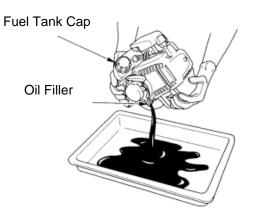
The recommended environmental temperature range of the machine is 5° to 105° F. We recommend the use of SAE 10W-30 engine oil, which equals to API classification SJ.
